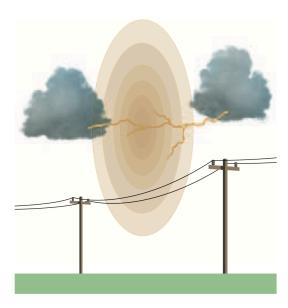
Transient overvoltages caused by lightning can reach magnitudes of 6,000 Volts in a well-insulated power distribution system. This is over 8 times the level tolerated by many electronic systems. Most importantly, lightning doesn't have to strike the building to cause destructive transient overvoltages.
