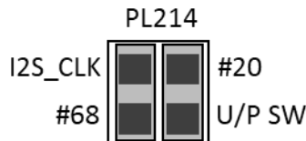
Figure 8: Default Jumper for PL214
